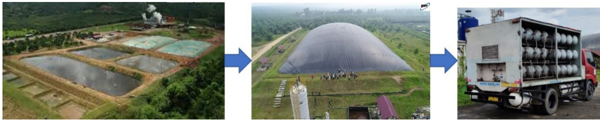
Figure 26 Schematic Illustration of POME Conversion to Biomethane for Fuel of Palm Oil Plantation Trucks 28
