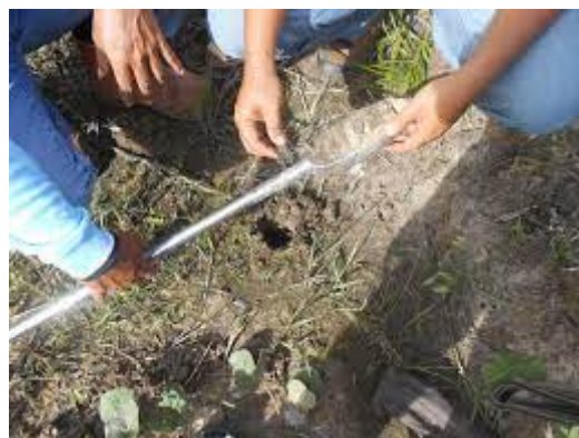
Figure 28 Soil Sampling Unit
